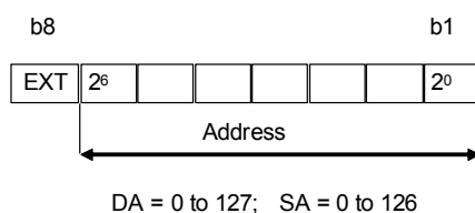
Figure 60 – Address octet coding
